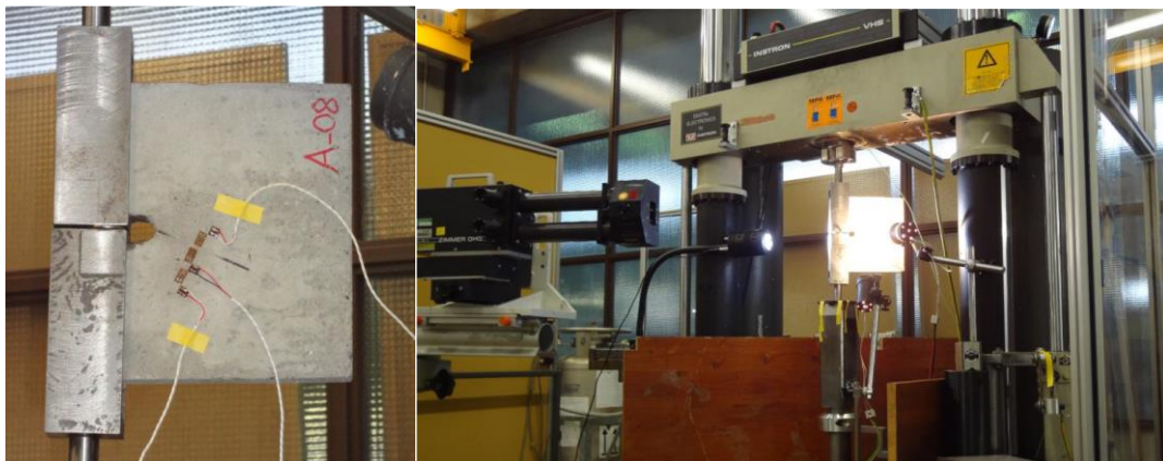
Figure 5-3. Strain gauges placed on the CT specimen and the experimental setup (Ruta, 2018).
