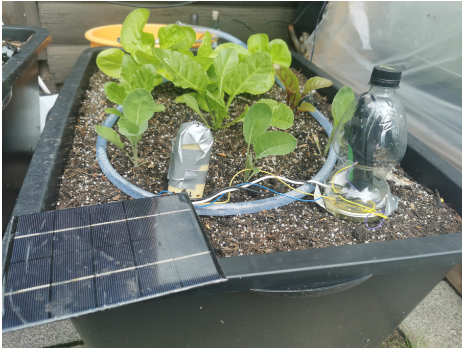
Figure 3.5: LILIGO Sensor with solar panel and battery
