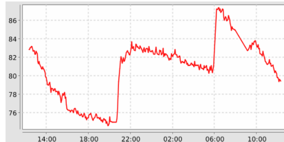
Figure 5.14: Using the script A.1 in Appendix A.3 Modify the Action Costs. The system watered at 21:00 and 6:00, as the solar radiation was below 30,000lx. Comparing with the other plots in this chapter: Without this script, the system often waters around 10:00 to 14:00, as this is the time, the moisture level usually falls below the MSL
