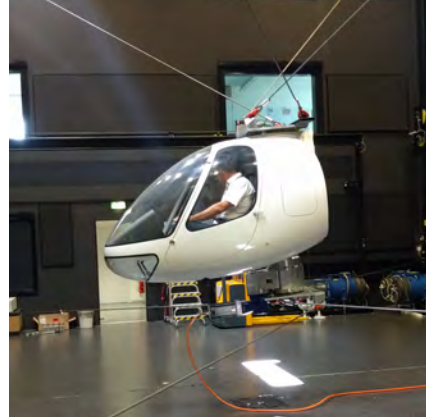
(a) Guimbal Cabri G2 Helicopter (A. Tarditi - (b) Guimbal Cabri G2 helicopter cabin mounted to the CRS. Hélicoptères Guimbal)
