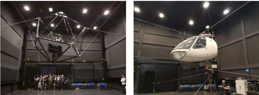
(a) The icosahedron shaped carbon fiber platform provides space for one or two seats while keeping the weight below 80 kg (b) The helicopter simulator uses a chassis from a Cabri G2 helicopter which is mounted to an endless rotating yaw-axis
