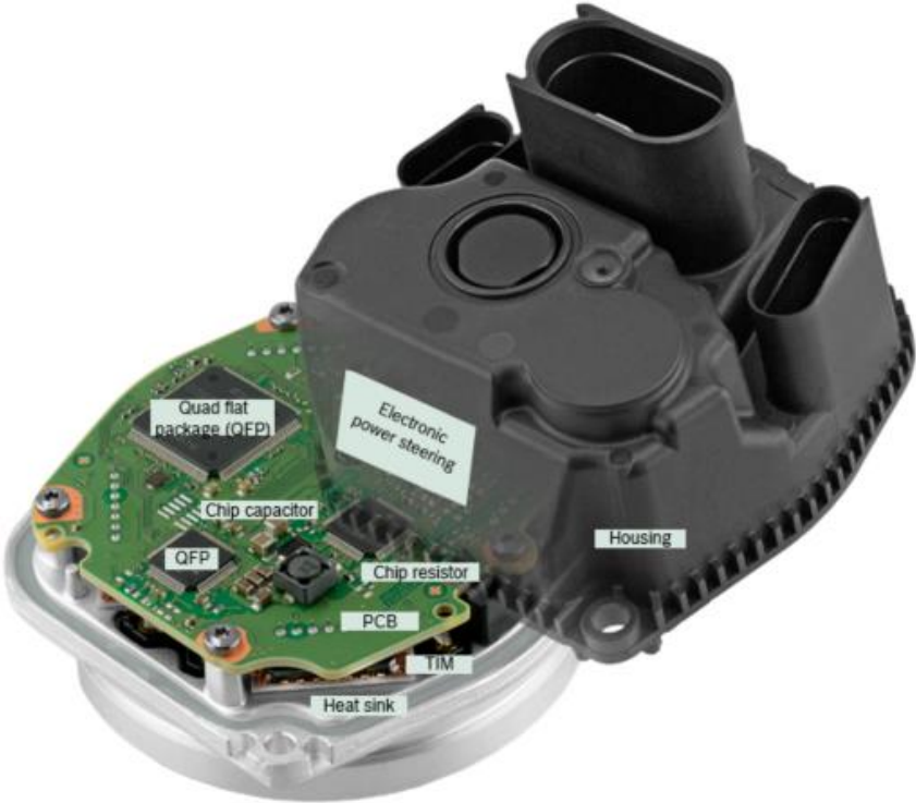
Fig. 1.2: Schematic configuration of electric power steering unit [2]
