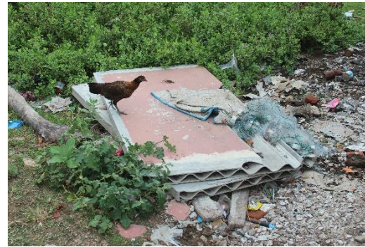
Figure 57. Panel containing asbestos on the ground, Banda Aceh. Source: Lucas, 2016.
