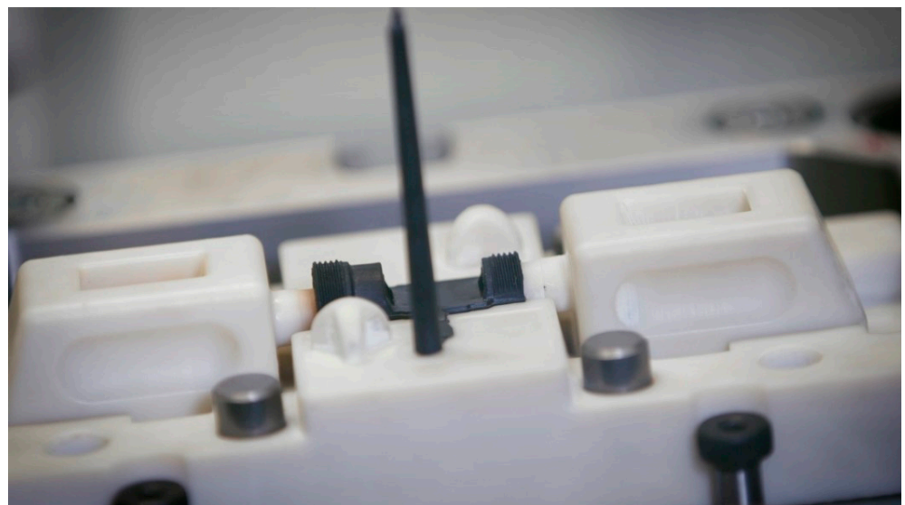
Figure 6. In-process injection molding with soft tooling with slides.
