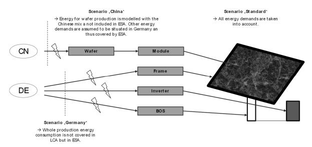
**Figure 5.** Schematic flow chart of the adjustment of LCA models in the use case for the adoption to ESA. The scenario *Standard* includes all energy inputs along the life cycle. The production groups include the module, frame, inverter and balance-of-system (BOS).
