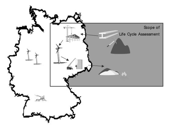
**Figure 2.** Graphical representation of the necessary adjustment in LCA for an integration into ESA with the geographical scope of Germany. Grey parts of the life cycle are included in the assessment; parts covered by the systems under investigation in the ESA are cut off to avoid double counting as the emissions are already covered by the ESA model.
