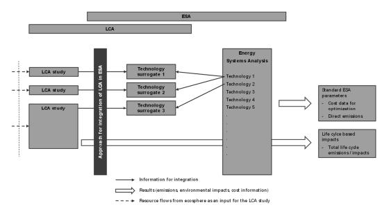
Figure 3. Schematic flow chart of the adjustment of LCA models for the adoption to ESA.
