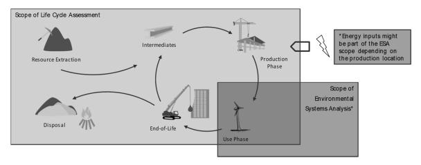
**Figure 1.** Graphical representation of the difference in the system boundaries for Life Cycle Assessment (LCA) and Energy Systems Analysis (ESA). LCA includes the environmental impacts from the whole life cycle, while ESA focuses on direct emissions from the use phase of, in this case an energy technology (energy inputs to other life cycle phases might be included depending on the production location).
