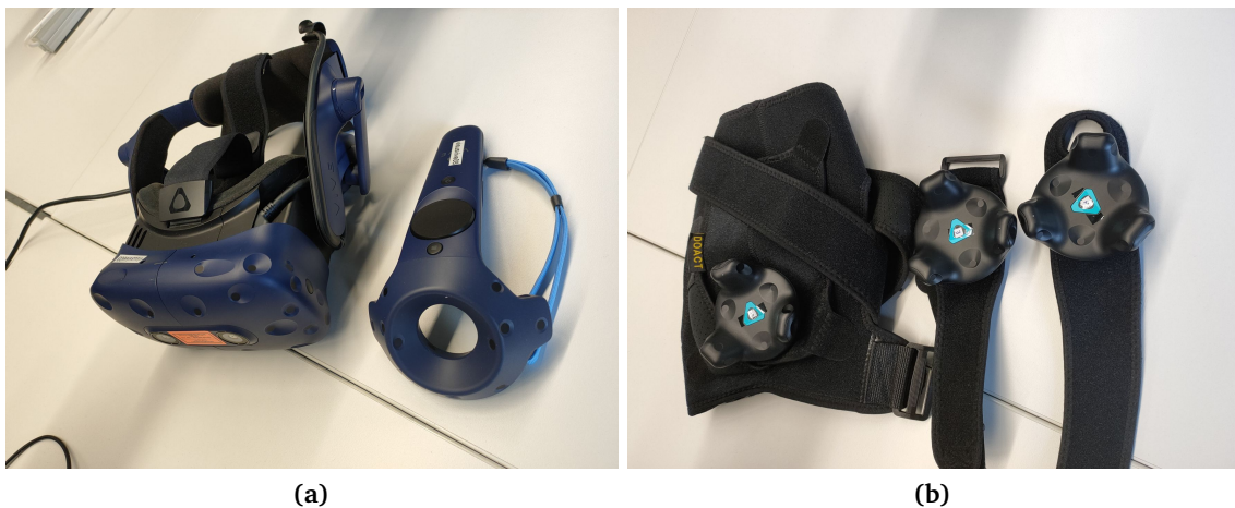
Figure 5.1: The hardware used for thesis a) The HTC VIVE VR glasses and the controller b) The VIVE trackers for the arms. On the left side the tracker for the shoulder, in the middle the tracker for the elbow and on the right side the tracker for the wrist
