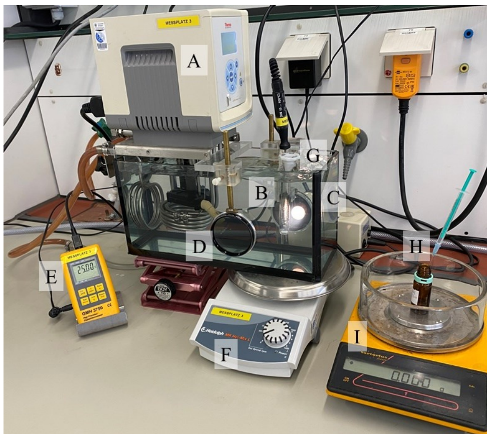
Figure 3.1: The house-built experimental setup for visual phase studies: A – thermostat, B – water basin, C – microscopy lamp, D – crossed polarizers, E – digital thermometer, F – magnetic stirrer, G – house-made sample holder with the sample, H – co-surfactant bottle with a syringe, I – balance for recording the amount of added co-surfactant.
