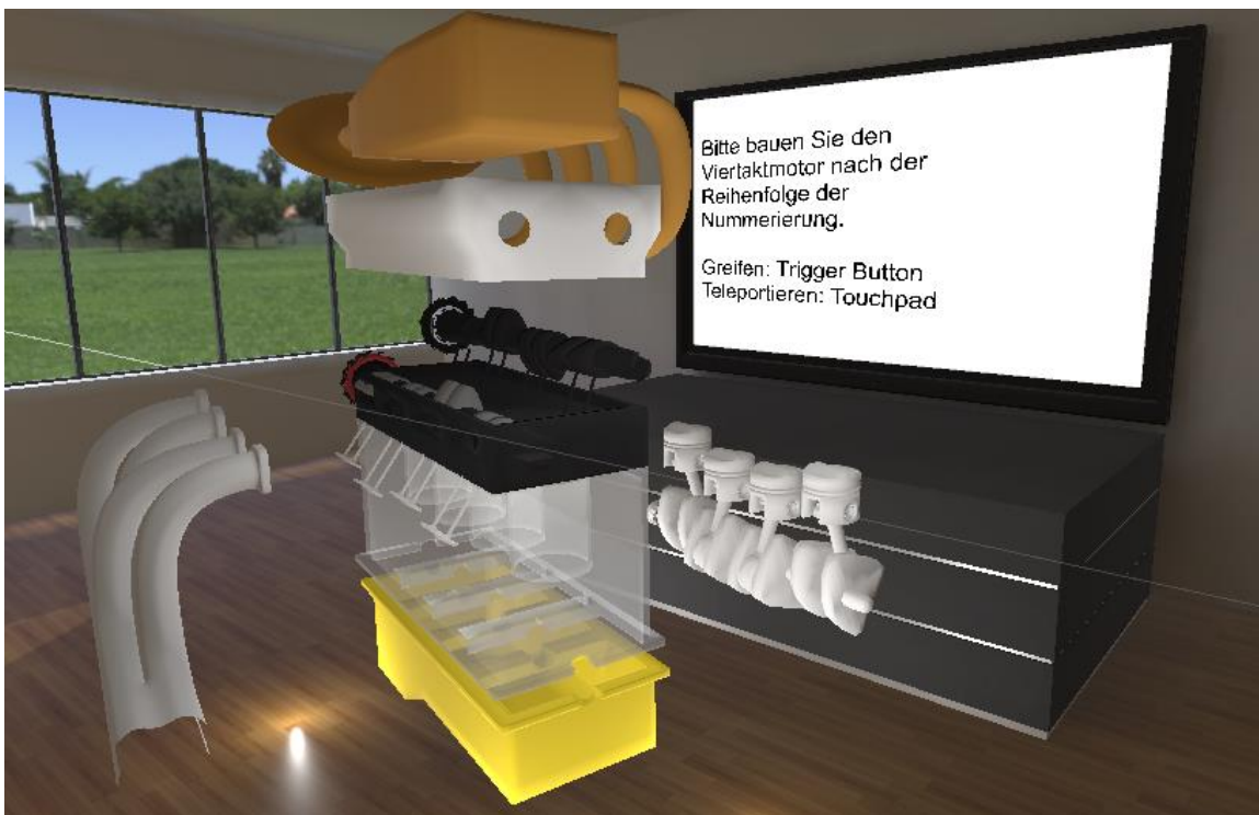
Figure 2-3 The learning scenario of the assembly of a four-stroke engine (source: own presentation)
