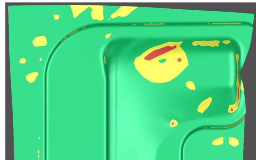
Figure 5-9: (a) Concept of the strain based UDV used in Chapter 8 for detecting “wrinkling initiation” and “developed wrinkling”; (b) defined colours for predicting wrinkling height in FEA
