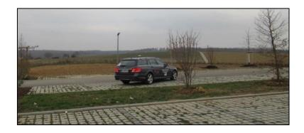
Figure 6-2: Test vehicle in the open-sky environment during the static measurement campaign. The antenna mounted on the rooftop is visible while the rest of the equipment is installed in the car (Avram et al. 2019)
