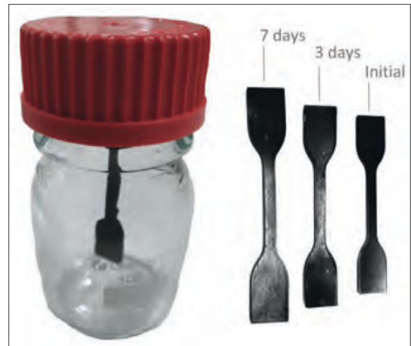
Figure 4: ISO 1817 submersion test of FPM dumb-bells ISO 37 type 2 (Fig.: IMA)
