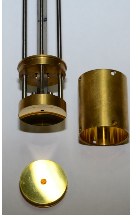
Figure 4.6.: Cavity part of the manufactured resonator made of brass. The sample can be placed in the center of the flat mirror. The casing connects the lower mirror with the upper round brass part which can be moved by a screw. The waveguide is made from steel to reduce heat conduction.
