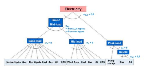
Figure A2. NEWAGE disaggregation of electricity generation.
