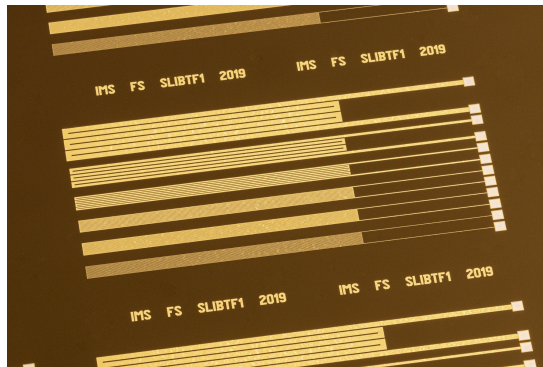
Figure 6.4: A zoomed view of a produced test foil
