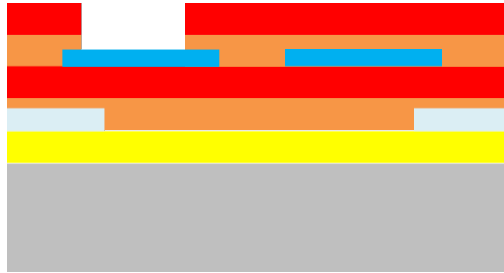
(i) Etching of BCB and PI for pad opening
