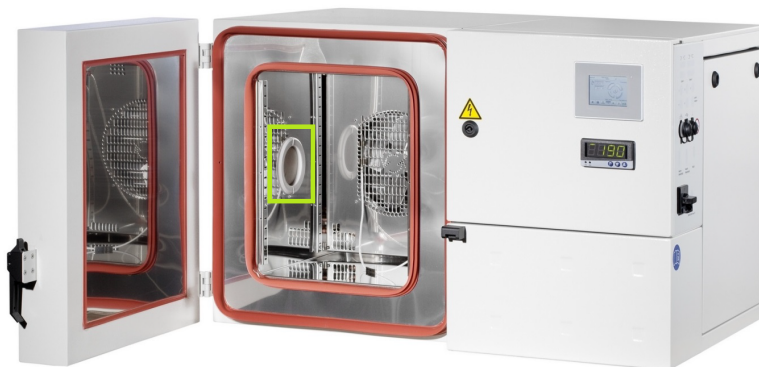
Figure 4.18: The Vötsch VT 4004 climate test chamber [93]
