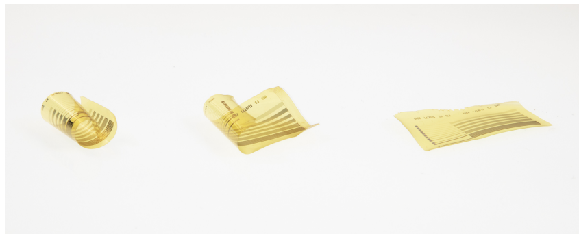
Figure 6.6: Test foils deformation of the 2-polymer process
