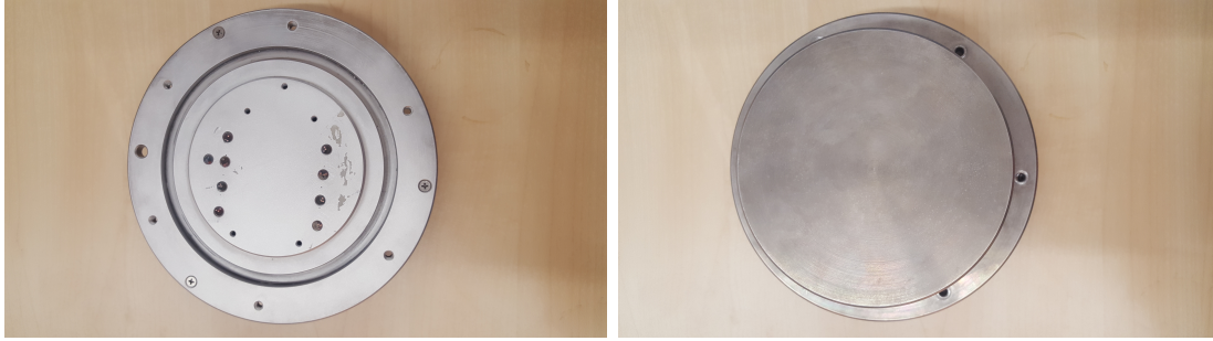
(a) Mounting threads for PCB
