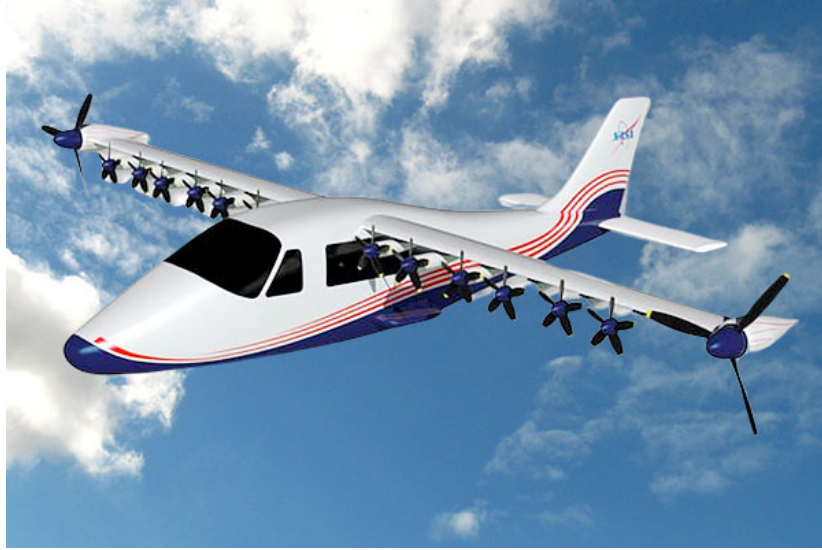
Figure 2.1: Aircraft concept "X-57 Maxwell" in its "Mod 4"-phase by NASA, image source: [22]
