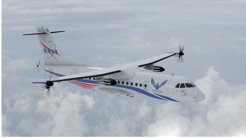
Figure 2.2: Preliminary aircraft concept "Parallel Electric-Gas Architecture with Synergistic Utilization" PEGASUS investigated by NASA, image source: [25]
