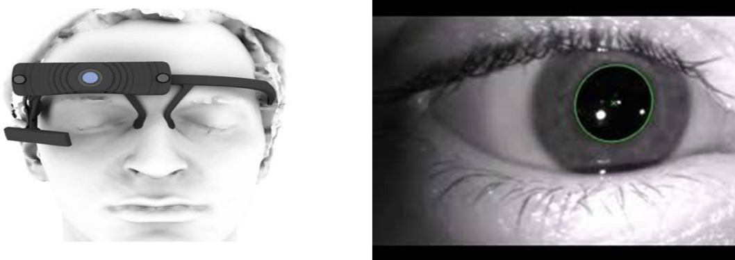
Figure 3.4: Pictures of wearing an eye tracker and the eye-camera view by Pupil Labs
