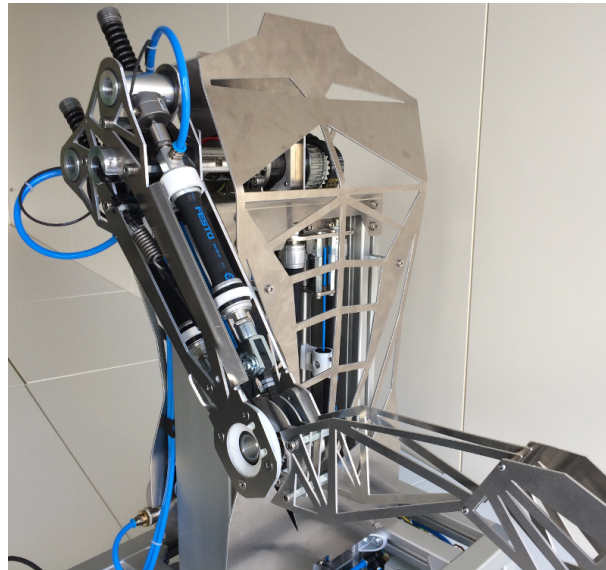
Figure 3.4: Real muscle-driven robot model mimicking the human arm model. The two joints (shoulder and elbow) are articulated by 5 pneumatic muscle spring units (MSUs), allowing movements in the sagittal plane. Two monoarticular MSUs drive each joint separately. The fifth MSU articulates both joints at the same time as a biarticular muscle to perform shoulder anteversion and elbow flexion [13].
