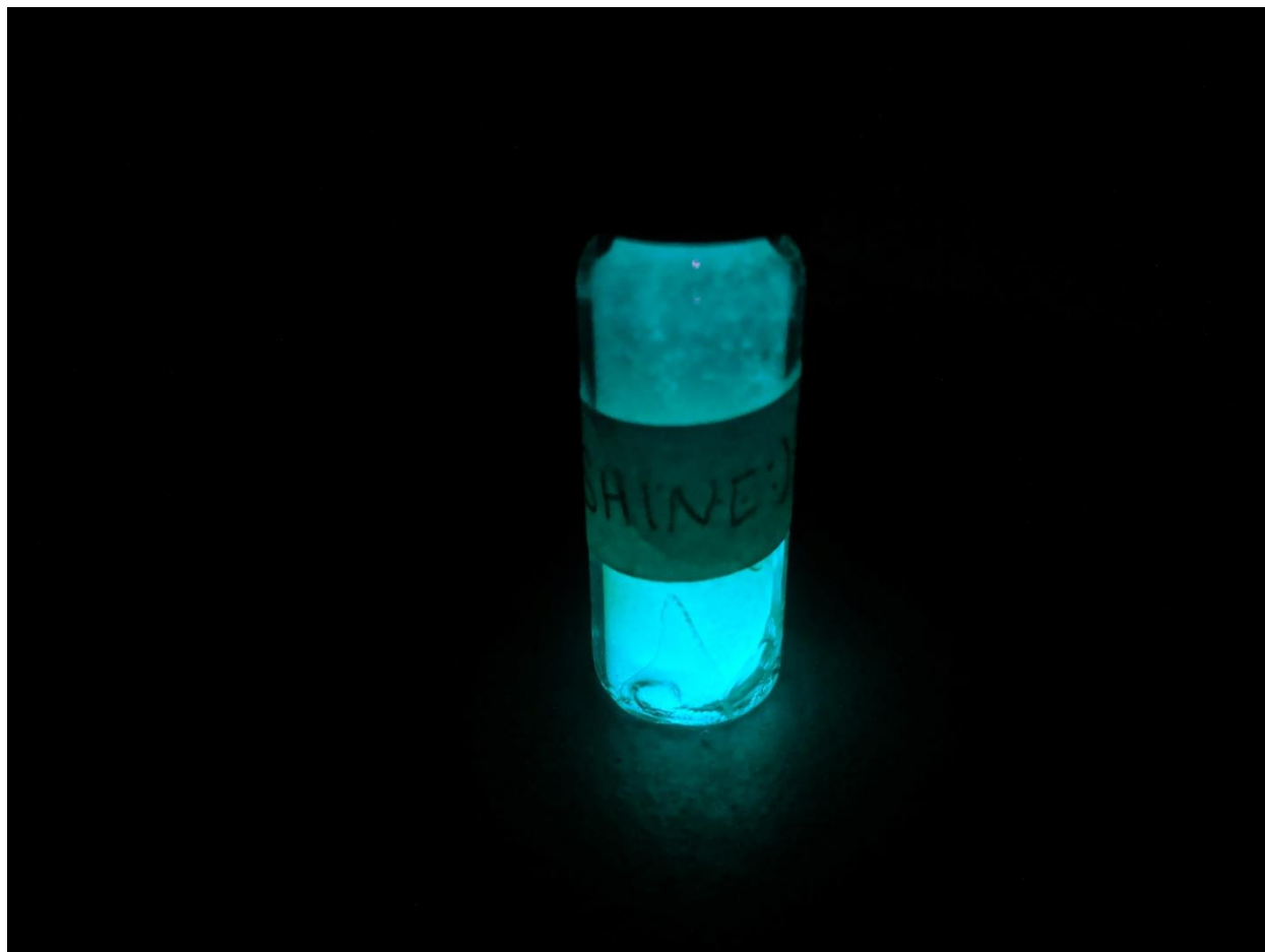
Scheme 147: Phosphorescing polyamide 6 synthesized at 200°C from a pre-homogenized (90°C, overnight) polymer system consisting of 400 equivalents AEO, 1 equivalent 5u-Me-CO 2 , 1 equivalent MgCl 2 , 1 equivalent AEO-Ac and about 5 to 10 wt.-% of an europium doped aluminum oxide received from lumentics.de.
