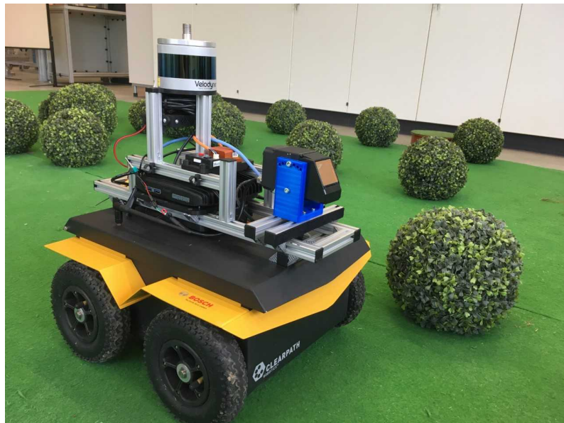
Figure 4.7: Jackal equipped with FX10 LiDAR
