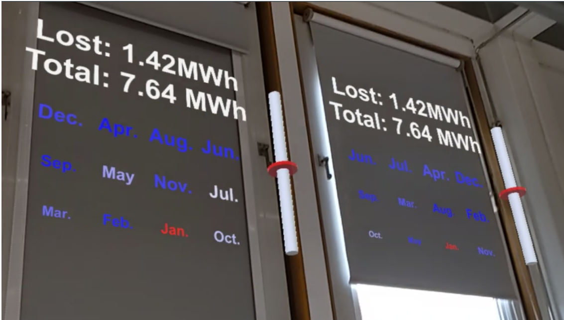
Figure 4.4: The final heat loss visualization. The size of the month names indicate the temperature difference. Months labeled red indicate that the window had a suspiciously low temperature difference and may leak. In this example, the window was open a lot in winter and summer, indicating too much heating or cooling
