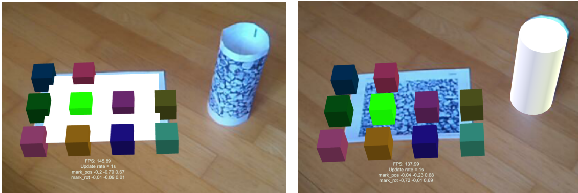
(a) Visualization bound to image marker, no offset is needed. (b) Visualization bound to cylinder marker. Offset is added in X and Z axes to make sure that the visualization appears outside the cylinder.
