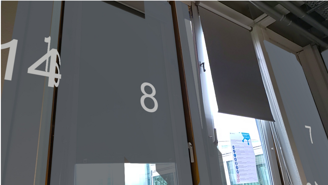
(a) Target selection using scene understanding to recognize surfaces. Notable is that only the left window is recognized properly, as the right window is tilted.
