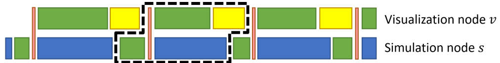
(c) Hybrid: Dynamic distribution of independent tasks between visualization and simulation nodes. Collective tasks are processed on visualization nodes only.
