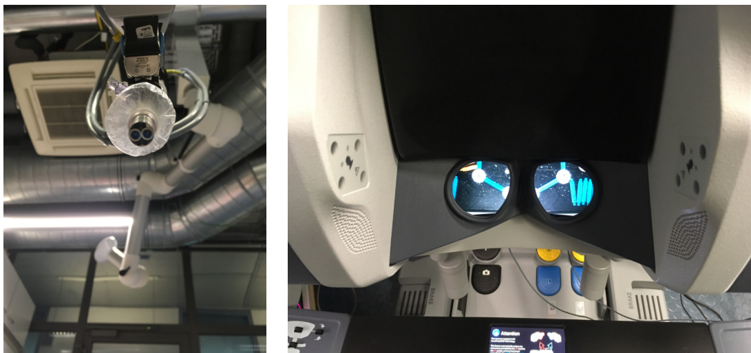
Figure 1.5: da Vinci stereo endoscope with stereoscopic vision. Left: Stereo endoscope. Right: Stereo viewer.
