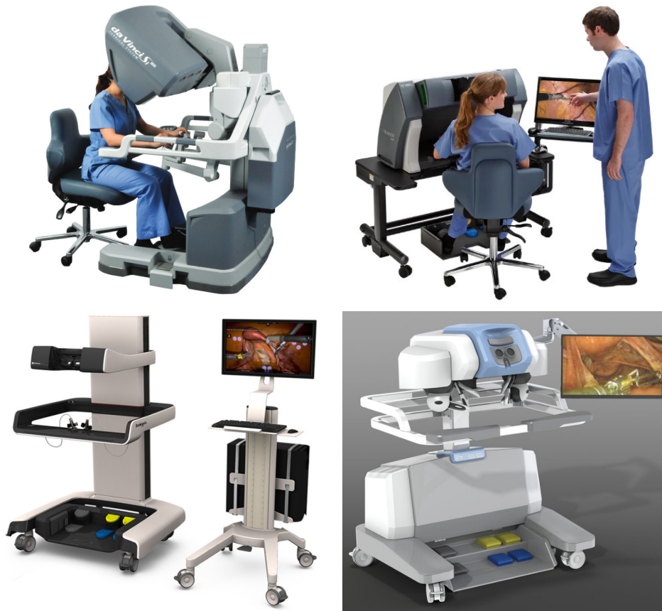
Figure 1.8: Common VR simulators. Top left: dVSS . Top right: dV-Trainer . Bottom left: RobotiX Mentor . Bottom right: RoSS . Adapted from Intuitive Surgical Inc., Mimic Simulation, 3D Systems formerly Symbionix, and Simulated Surgical Systems [Simb; Simc; Sur; Sys].
