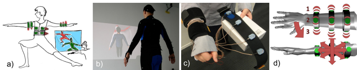
Figure 2.7: Multimodal motion guidance system. a) Haptic feedback to guide user motions for following remote teachers. b) Motion capture. c) Vibration actuators. d) Concept of haptic feedback for motion guidance regarding direction and speed. Reprinted from Schonauer et al. [SFO+12].
