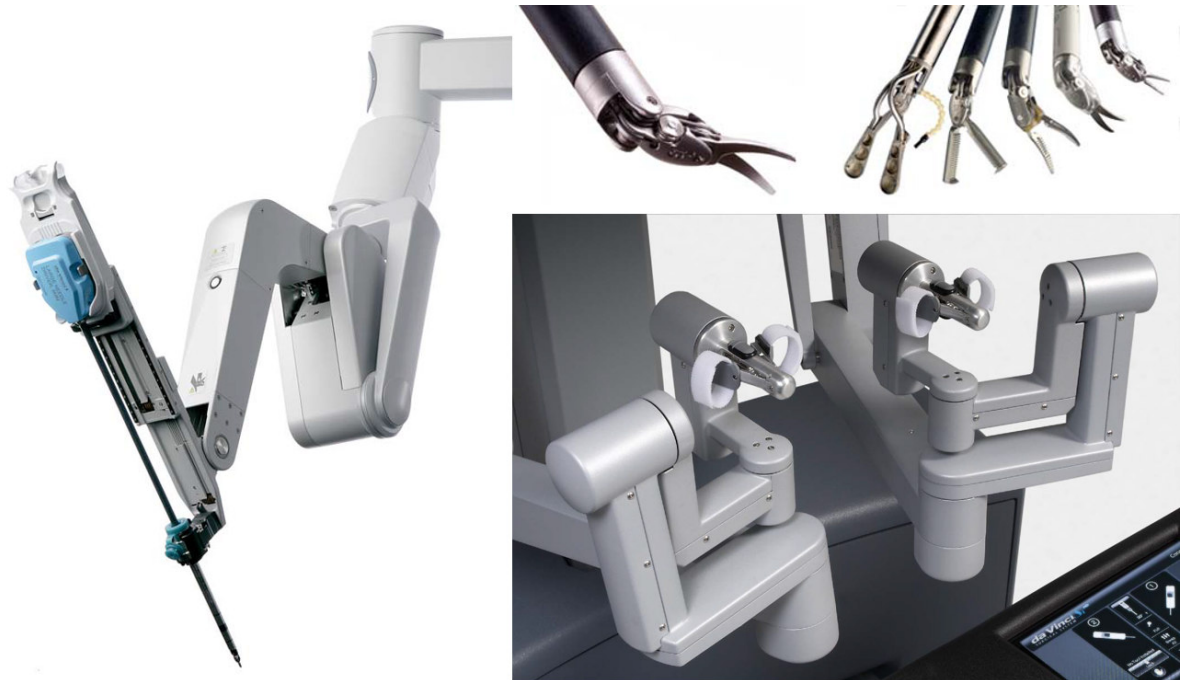
Figure 1.4: da Vinci instrument arm with EndoWrist instruments and surgeon handles. Left: da Vinci instrument arm with attached EndoWrist instrument. Top right: EndoWrist instruments. Bottom right: Surgeon handles. Reprinted from Intuitive Surgical Inc. [Sur12].
