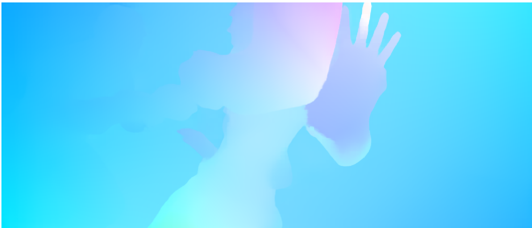
(B) Color representation of the optical flow of the frame as calculated by RAFT.
