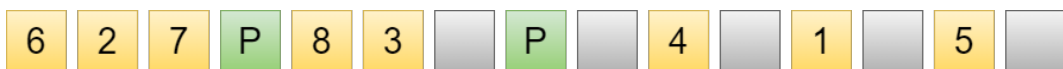
Figure 6.3: Configuration creation order of the DivideAndConquer strategy. (P: created in the preparation phase)
