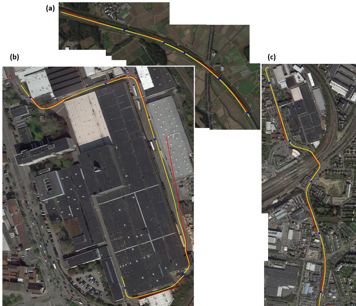
Figure 6.11: Path approximations provided by combined scan point sampling strategies (yellow) compared with odometry-only reconstruction (red): (a) combine3 , (b) combine2 , (c) combine1 . Map data: Google, ZENRIN, GeoBasis-DE/BKG.
