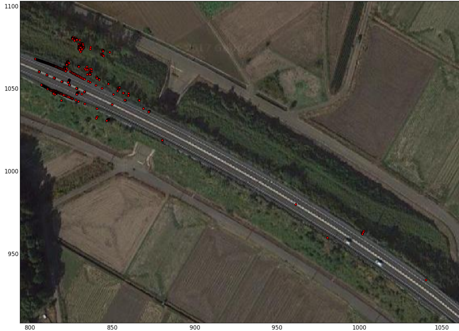
Figure 6.1: Scan point cloud aligned to satellite imagery. Map data: Google, ZENRIN.
