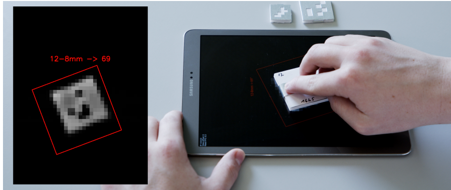
Figure 6.1: This sample application displays the capacitive matrix, including the blob boundaries, current classification result, and rotation prediction of fiducial tangibles on the screen.
