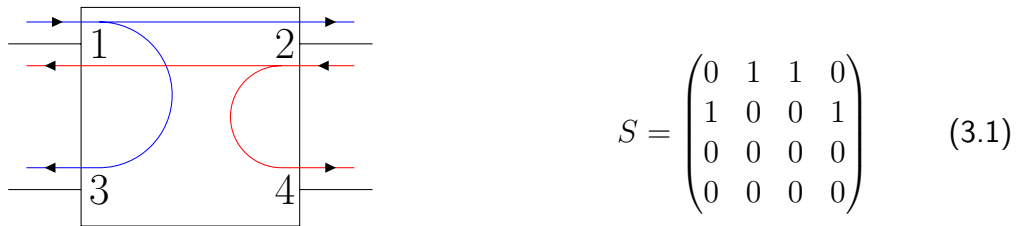
Figure 3.2.: Block diagram of the equation-based S-parameter block (left) used as ideal coupler with its S-parameter matrix (right).
