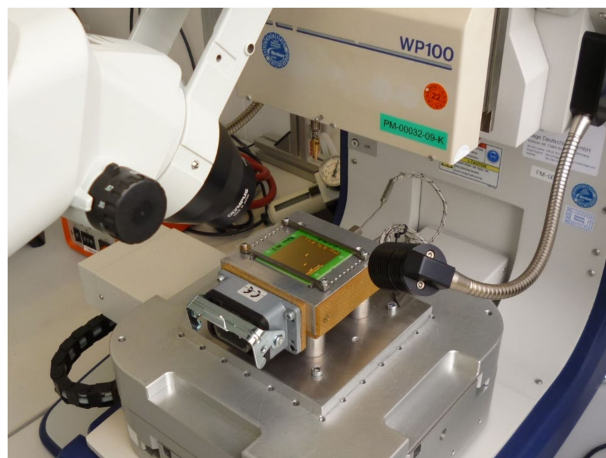
Figure 5. Test setup for pull tests by Nordsen DAGE 4000 plus.
