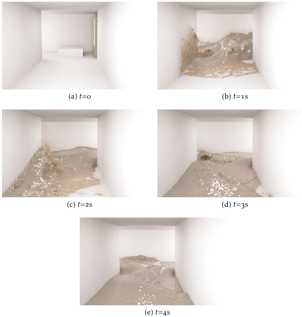
Figure B.2: Dam break simulation with 1 million particles with direct raytracing of an isosurface with motion blur and global illumination. Frames in 1 second steps.
