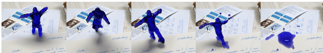
Figure 3.2: SPH simulation coupled with an IK skeleton. Background image with friendly permission for this usage from Andreas Nilsson [73]. A video sequence of the animation can be found in the video appendix [63].
