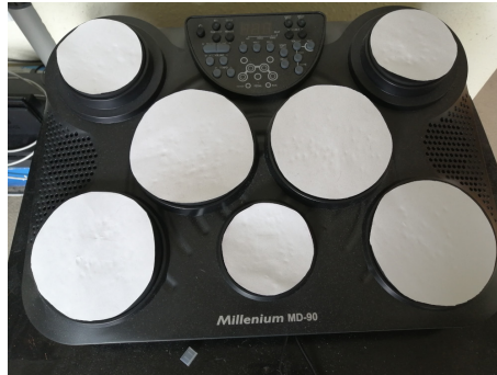
Figure 3.2: E-drum kit with white paper stuck onto the drum pads to improve the visibility of the projections.
