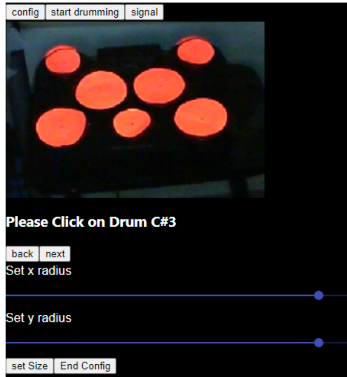
Figure 3.4: User interface to manually track drum pads. Users can go back and forth to a list of all drums and set their locations by clicking on the center of the corresponding drum on the webcam picture. They can then set the desired size of the ellipses via the sliders on the bottom.
