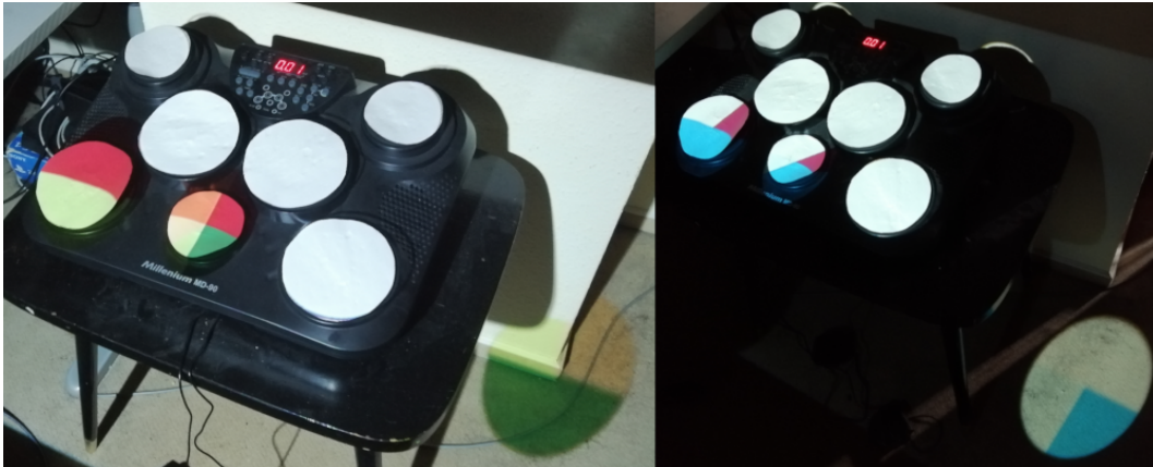
Figure 4.10: Implementations of pie chart visualization. We tried visualizing how accurate notes were played from perfect to miss (left), and visualizing how many notes were played too late, too early, or perfect (right). We decided to use the latter implementation because we believe this information is more useful.
