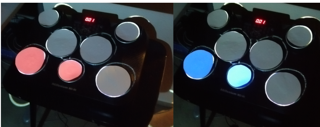
Figure 4.11: Signal visualization implementation. When the user is too slow, the drums are colored red (left), when they are too fast, the drums are colored blue (right).
