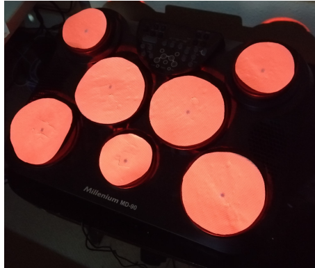
Figure 4.1: Ellipses are projected onto the drums right as their positions are set, to help users more easily find the center. Black dots show the coordinates the user clicked.
