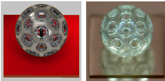
FIGURE 1.1. Hollow buckyball with rod structure inside. CAD model (left) and 3D printed part produced with femtosecond two-photon 3D printing (right). The diameter of the printed buckyball is 400 \mu\text{m} .
