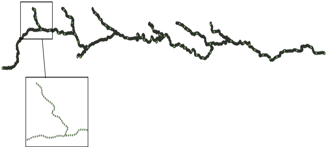
Figure 3.3: Node product for the Po River. Node product is with mean values around each node for parameters such as width, height, flooded area, etc.
