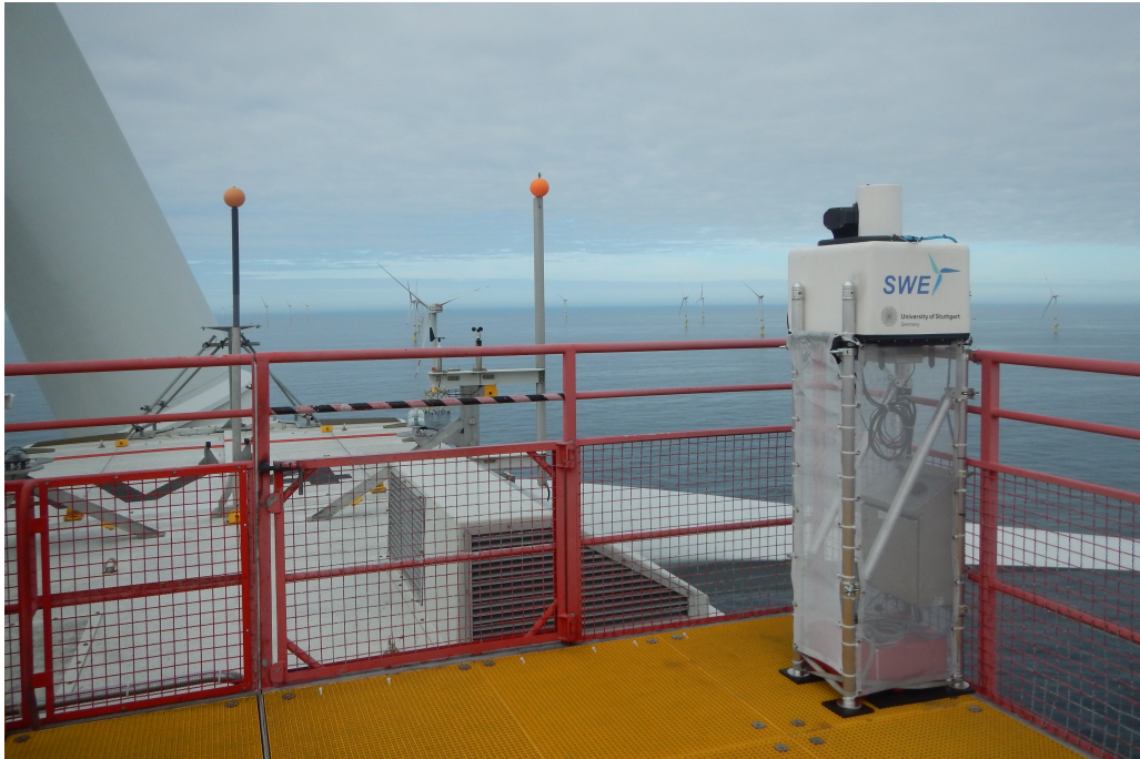
Figure 4.6: StreamLine XR lidar on the nacelle of the AV04 turbine in alpha ventus.
