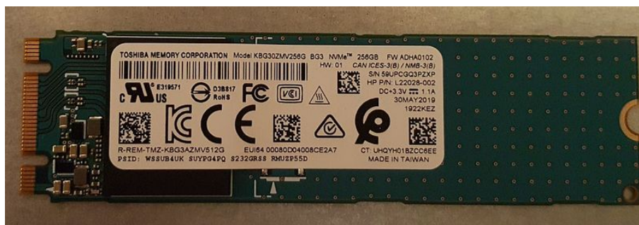
Figure 4.2: The M.2 NVME SSD used for Windows 11[10]
