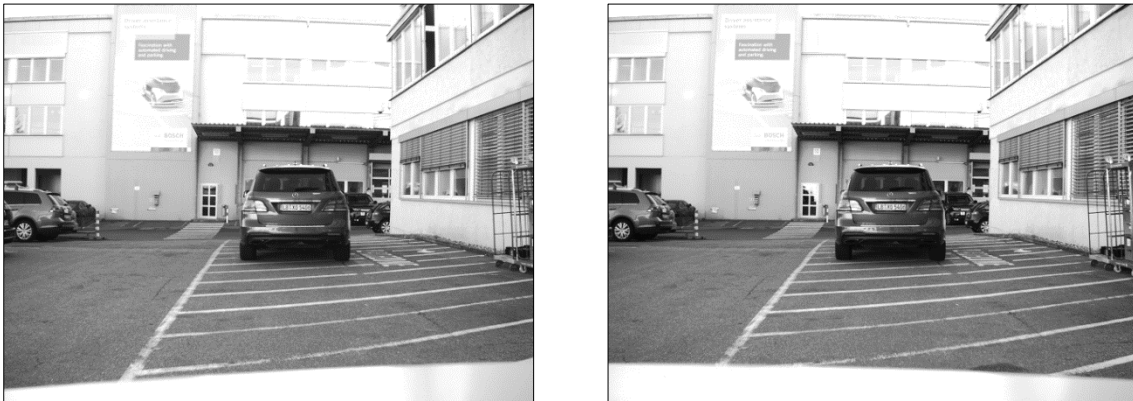
a b Fig. 7.9. Stereo image pairs taken from a front vehicle using a stereo front-view camera The distance of the vehicle to the camera is around 10 [m] a: left image, b: right image (Courtesy of Robert Bosch GmbH)
