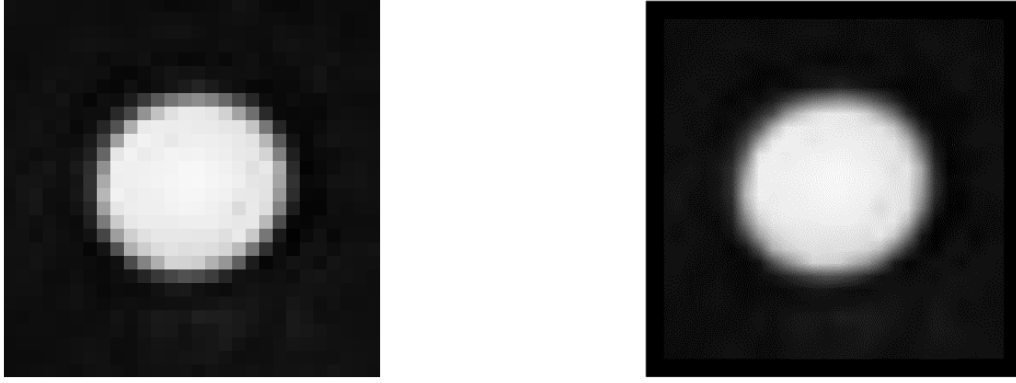
a B Fig. 2.33. Sub-pixel sampling and Sub-pixel interpolation a: Example of a visible marker in image b: Sub-pixel sampling using Gaussian anti-aliasing filter, Sub-Pixel depth = 0.1 [Pixel] (Courtesy of Robert Bosch GmbH)
