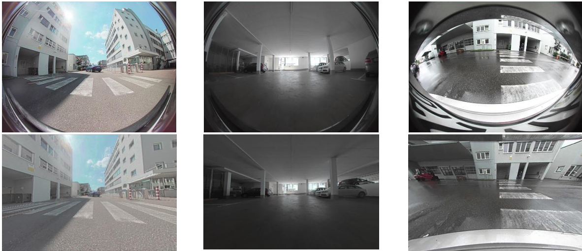
Fig. 3.5. Image rectification using the C2W (2D-3D) and W2C (3D-2D) transformations a, b, c: original images from an omni-directional camera installed in vehicle d, e, f: rectified images corresponding to the above images respectively (Courtesy of Robert Bosch GmbH)
