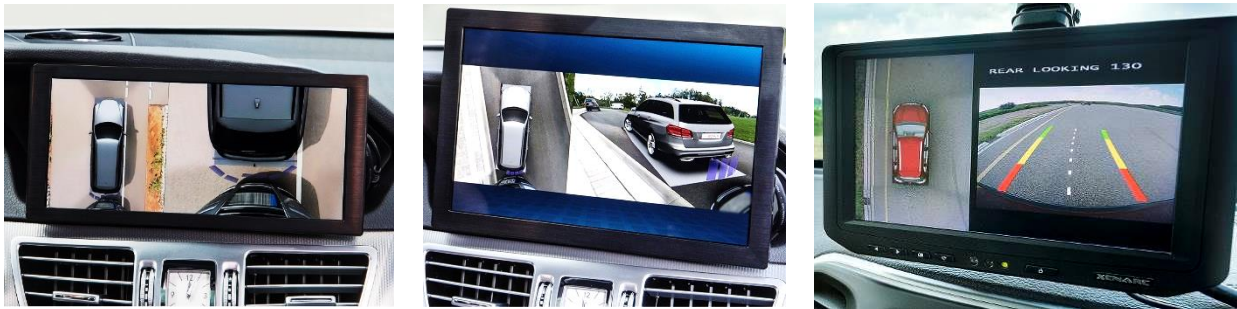
a b c Fig. 2.13. Examples of Driver-Assistant Applications a: 3DTV: top and trailer view b: 3DSV: top and rear-to-front view c: 3DTV: top and rear view (Courtesy of Robert Bosch GmbH)
