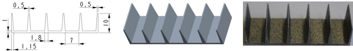
Figure 6-10: Technical drawing of ribs geometry on support with dimensions in mm (left); CAD view (middle); aluminium ribs 3D-printed using selective laser melting (SLM).
