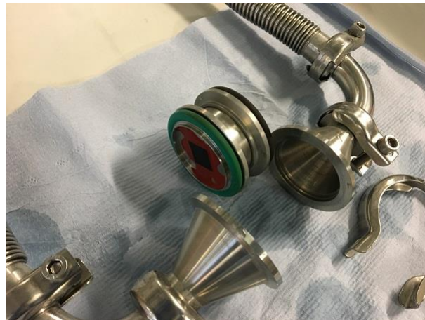
Figure B-4: Permeation cell with two commercial, identical consolidated activated carbon composites in series ( GAP_1 and GAP_2 ).
