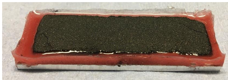
Figure C-1: CDC composite containing 2 wt% CMC binder ( EXP_{CDC} ) attached by means of thermal adhesive tape on a 2 mm thick aluminium support with a horizontal slit for the thermocouple.
