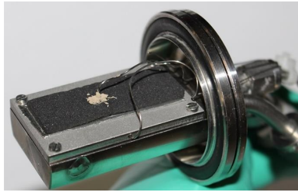
Figure 4-6: Sample holder for the equilibrium plant consisting of the temperature-controlled sample holder, metal plate, thermocouples, and consolidated CDC-composite.
