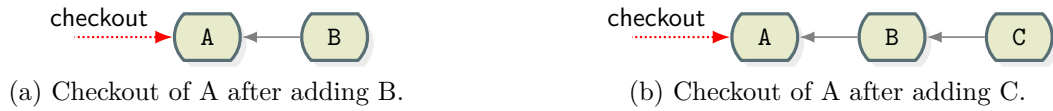
Figure 3.3: The checkout of A must lead to the same output in both cases.
