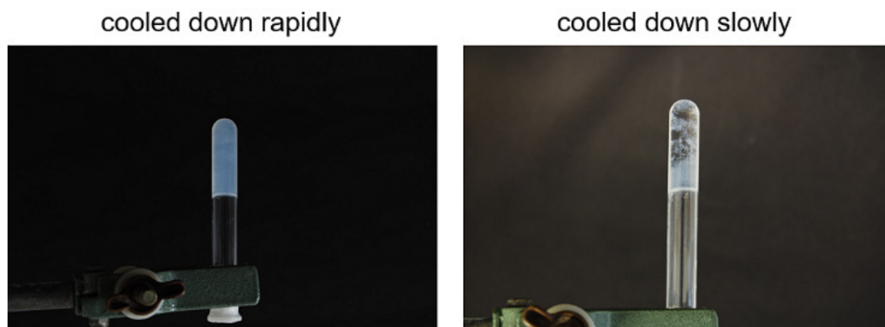
Figure 4.4: Comparison of a gelled lamellar phase cooled down either rapidly ( left ) or slowly ( right ).
