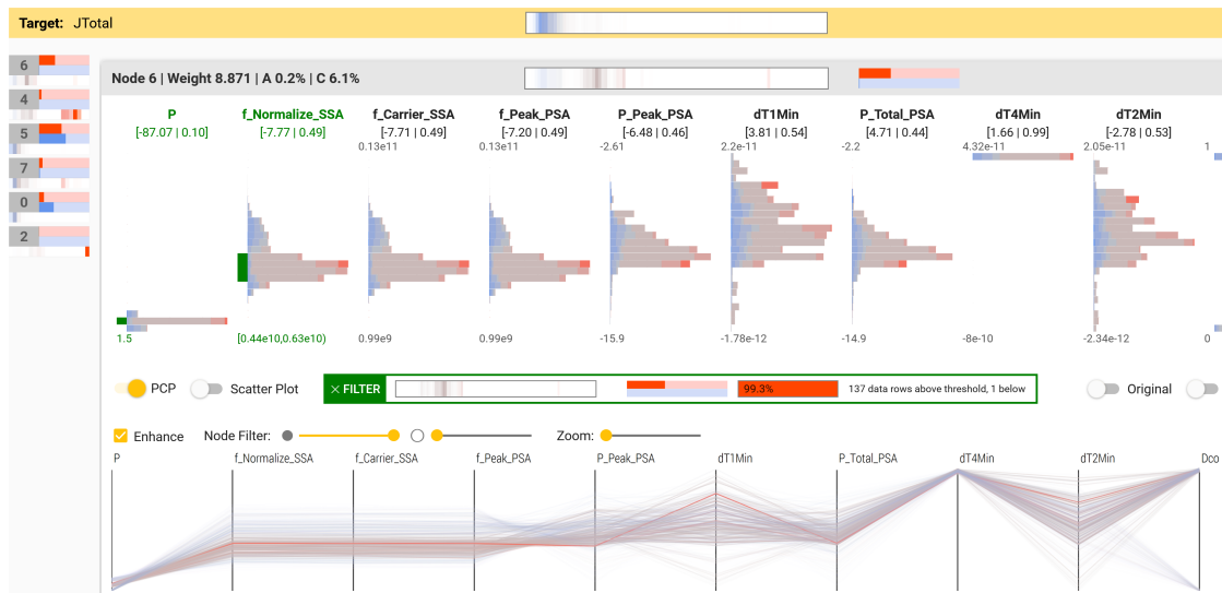
Figure 7.3 — Visual Neural Decomposition of a chip testing measurement data set with the goal to identify cases in which the target variable (here: jitter) exhibits high values. Each node visualizes parts of the data set depending on its activation.
