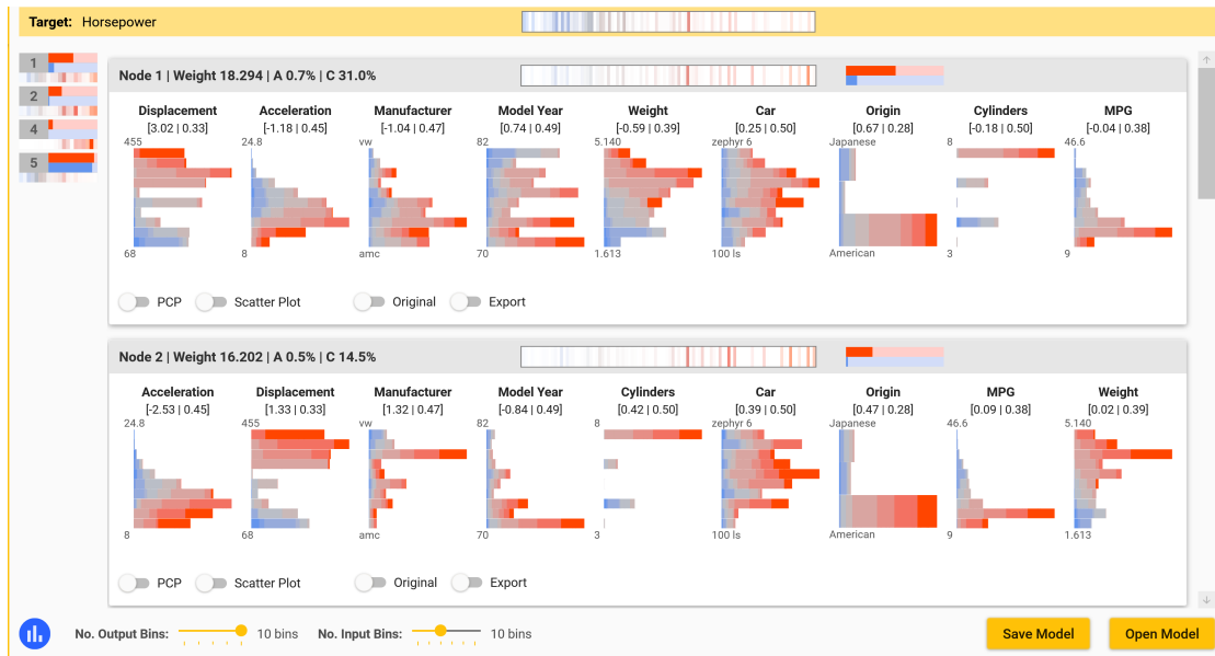
Figure 7.6 — Visualization of the resulting model. Each card represents one hidden node and visualizes the data set filtered by the contribution of the respective node. A compact overview of the nodes is shown on the left.
