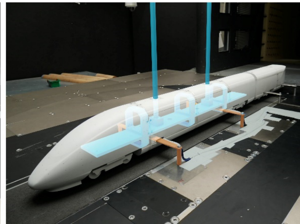
Figure 4. Model supports: (a) Model, crossbeams and struts are connected to the underfloor balance, (b) only the crossbeams and struts are on the balance, the train car model is supported by the wind tunnel’s manipulator.
