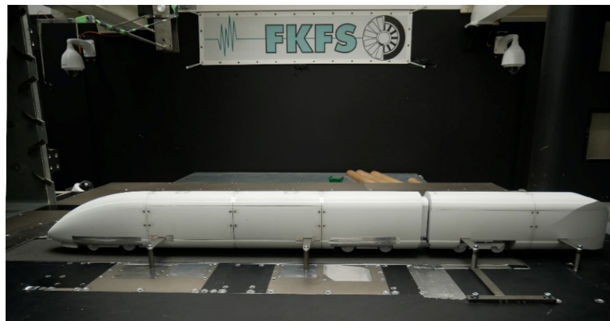
Figure 3. A 1:20 scale model in the IFS model scale wind tunnel of the University of Stuttgart, positioned according to the true flat ground configuration.
