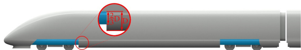
Figure 2. Geometry of bogie fairings (D: height of the bogie cutout).
