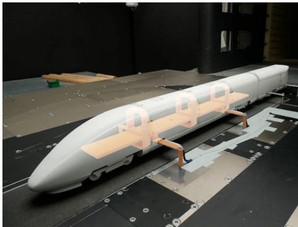
Figure 4. Model supports: (a) Model, crossbeams and struts are connected to the underfloor balance, (b) only the crossbeams and struts are on the balance, the train car model is supported by the wind tunnel’s manipulator.
