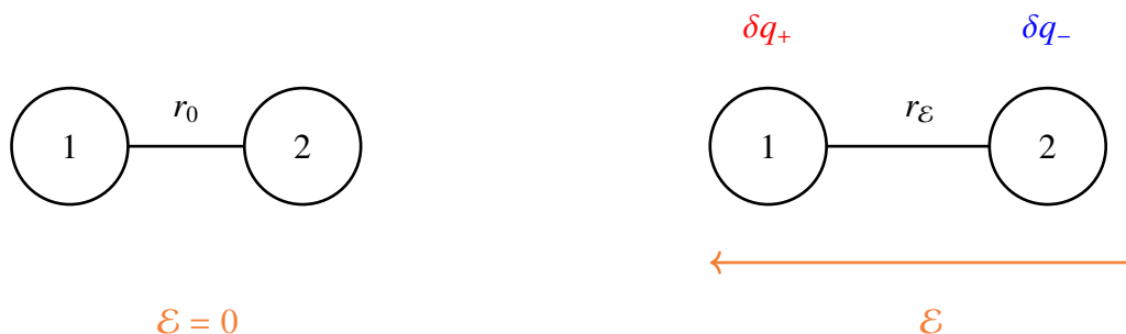
Figure 3.6: Schematics of possible charge shifts in a homo-nuclear dimer. The total charge shift between the two atoms is indicated with \delta and can be observed in the simulation via partial charge calculations. The length of the equilibrium geometry before and after field application is indicated by r_0 for the field free case and r_{\mathcal{E}} in the presence of fields.
