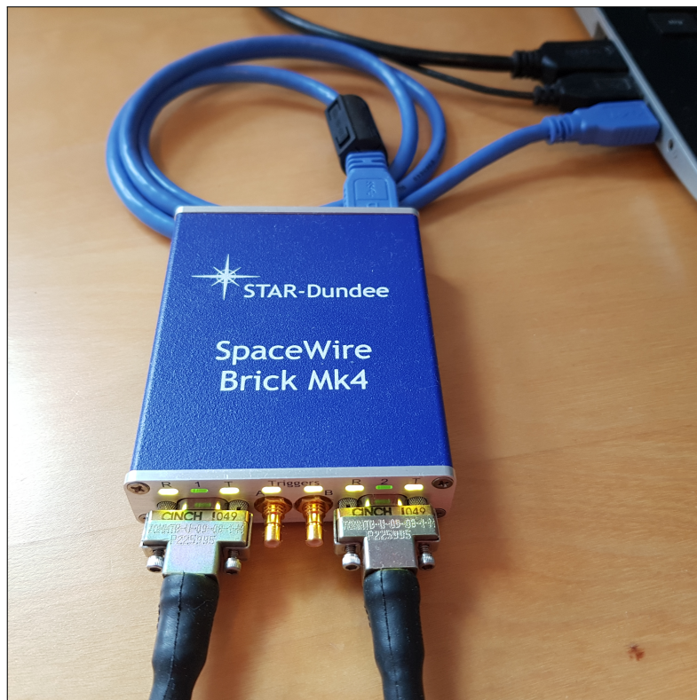
Figure 10: Hardware setup; top: USB cable to PC; center: Brick Mk4; bottom: SpaceWire loop
