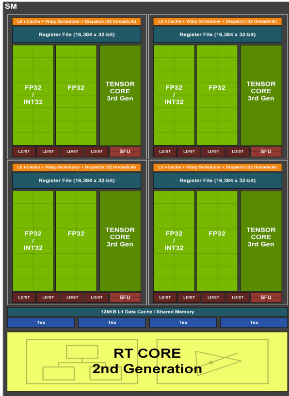
Figure 4.1: A single SM multiprocessor of the GA102 architecture. The SM is a composition of four partitions and shared memory. Every partition has floating-point, integer, load-store, and special function units. Every SM partition has a shared instruction counter, a local register file, and a small shared instruction cache.
