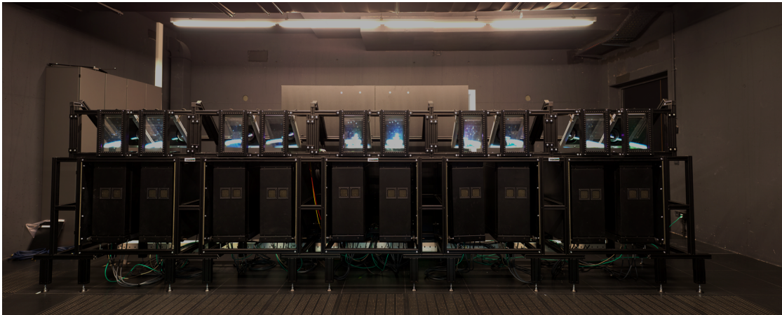
Figure 2.3 — The projector array of the stereo capable large high-resolution display at VISUS 1 . The ten projectors are divided up into two groups, five project the left and the other five the right eye of the stereo image. They are placed on a metal framework that allows to move each projector individually in order to align them to get an image without holes. © VISUS
