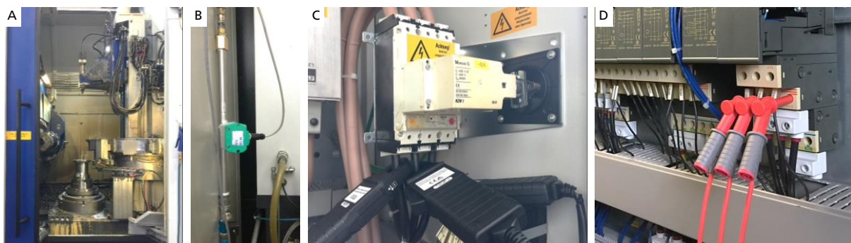
Figure 2-10 Example of an energy metering setup in a milling center. (A) – machine tool, (B) – compressed air flow measurement, (C) – current collectors installed on the main switch of the machine tool, (D) – voltage reference
