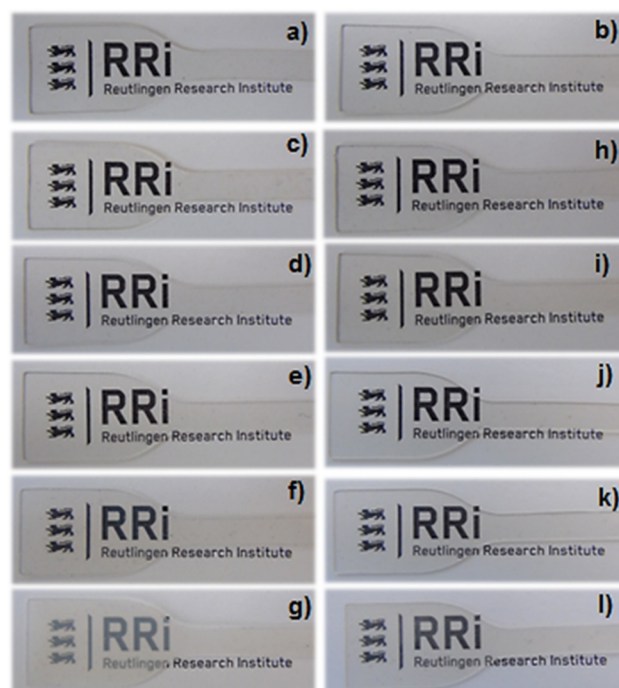
Figure A5. Photographs of PDMS-based PUr elastomer samples used for tensile testing. (a) PSU MDI-1.5%. (b) PSU CHDI-1.0%. (c–g) PSU H 12 MDI series with HS contents: (c) 1.6%, (d) 5%, (e) 10%, (f) 15%, and (g) 20%. (h–l) PSU IPDI series with HS contents: (h) 1.4%, (i) 5%, (j) 10%, (k) 15%, and (l) 20%. All PSU elastomer films were transparent until a HS content of 10%. The PSU elastomer films became translucent at HS contents of 15% and 20%.
