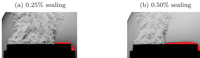
Figure 5.10: Schlieren images to illustrate outflow behaviour of coolant (here helium) for partial sealing of porous sample (red areas illustrate sealing by adhesive)
