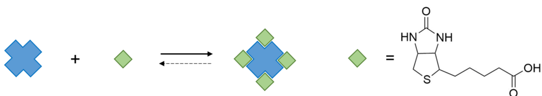
Figure 2.14: Schematic drawing of the biotin-(strept)avidin interaction (left), chemical structure of biotin (right).
